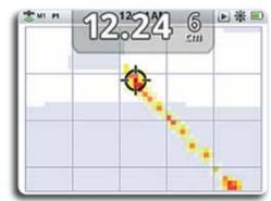
Target Trace displays many detections per second to offer greater visual detail of a target's identity. Multiple targets are displayed as coloured 'hot spots', or streaks, across the Detect screen – turning everyone into experts. Choose to have on or off while detecting or during pinpointing.
