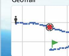
A GeoTrail is a coloured trail on the Map screen which shows where you have been detecting. You can be confident that no ground has been left unsearched. The GeoTrail changes colour when being recorded as part of a GeoHunt.
