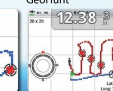
A GeoHunt is made up of your GeoTrail and any WayPoints and FindPoints you mark along the way. A GeoHunt is displayed on the Map screen and can be placed onto Google Maps to record your successes and plan your next hunt. Ten GeoHunts can be stored in the detector.
