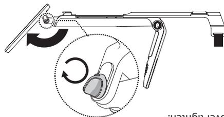
**STEP 4.** Fold out the search coil to detect parallel with the ground (Refer to 'Detecting Basics'). Tighten the nut to fix the coil position. Be careful not to over tighten.
