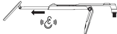
**STEP 5.** Fully extend the lower shaft until you hear it click into place. To retract shaft, firmly tap on the base of the coil.
