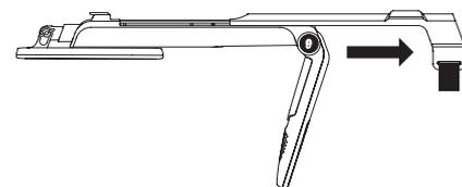
**STEP 3.** Slide out the armrest to desired length (typically just under your elbow).
