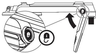
**STEP 6.** Release the camlock lever to adjust the upper shaft to desired length, for your height (Refer to 'Detecting Basics'). Close the camlock lever to lock into position.
