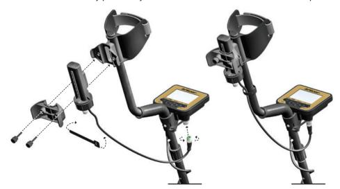
The battery pack takes 4 AA Alkaline or rechargeable NiCd or NiMH batteries.
